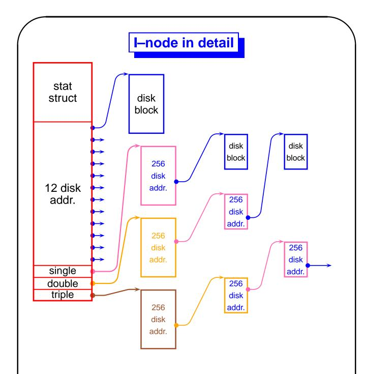
How many disk addresses fit into a disk block depends on the size of an address and on the amount of additional information stored. The number shown, 256 is a common case. The format of a block group and I-node shown are for the standard linux file system ext2 (also used in ext3).
