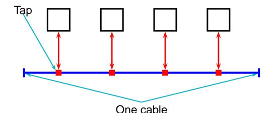
A **tap** is a passive transceiver (signal passes by through the tap unchanged).
