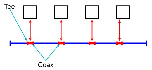
A BNC tee captures the signal and sends (all of it) to the station's NIC. The NIC has to regenerate the signal (note the reliability issue).
