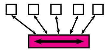
In its simplest form, the hub relayed all of its input (from all ports) to all of its port (excluding the source port). Fancier variants exist.
