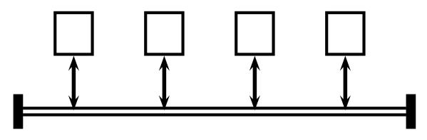
The link was designed as a single bi–directional channel, typically a coax cable. Soon two unidirectional links were used instead (see twisted pair) and the bus architecture was replaced by hubs.
