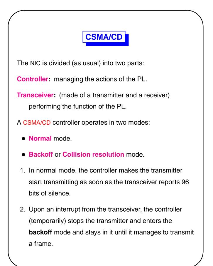
Note that when a single node is interested in transmitting a large file, CSMA/CD is always in the normal mode and its efficiency approaches  $\frac{1500}{1500+26+96/8} = 97\%$
