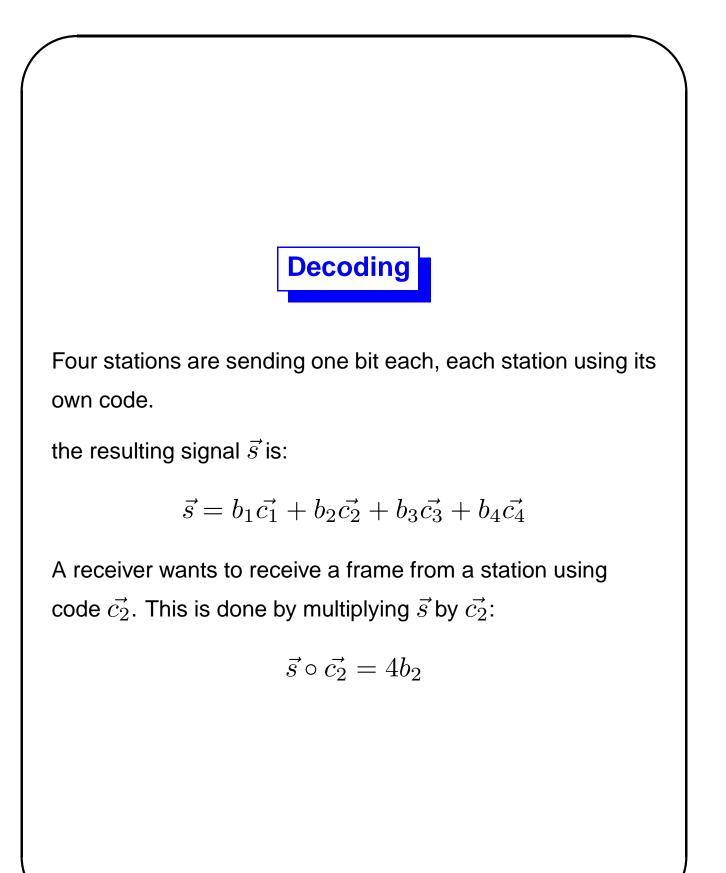
In reality it is not feasible to give truly orthogonal vectors (the different components of the signal will show at the receiver at slightly different times). So, a certain degree of noise will show as a result of the multiplication done by the receiver.
