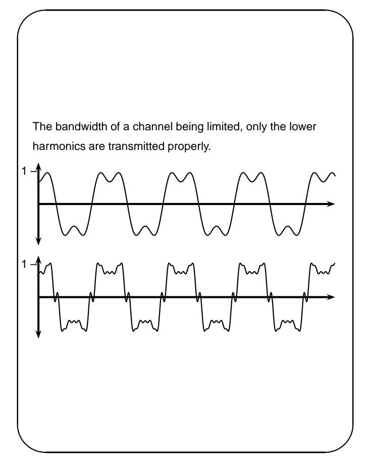
Digital signal of rate 500 b/s is to be transmitted over a link. Derive the minimum bandwidth required (in Hz). The worst case is the sequence of alternating 0's and 1's which has a fundamental frequency of 250 Hz (2 bits per period). The harmonics are: 750 Hz, 1250 Hz, 1750 Hz, etc. Hence the minimum bandwidth is 0–250 Hz for the fundamental frequency only, 0–1250 Hz for the  $\omega_0 - 3\omega_0 + 5\omega_0$ , etc.
