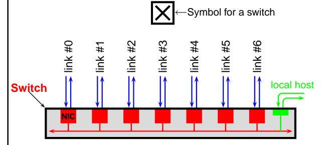
Several bi-directional links ("interfaces") are connected to a switch; each link is handled a device that resembles a NIC card in a computer.
