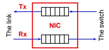
This makes access to a switch collision—free but introduces the possibility of frames being dropped inside a switch due to congestion (contention for output buffers or for internal interconnection).
