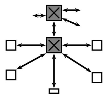
Switches can be connected to other switches, creating a WAN with Data Link Layer "routers" (switches). The main difference (besides the obvious absence of IP) is that switches do not know whether a link leads to a switch or to a host. Therefore they do not exchange information. Likewise, switches do not choose the path for a frame—it is automatically given by their tables.
