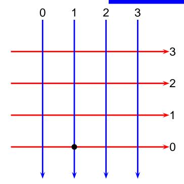
If (1) sends a frame to (0), input bus 0 will pick the frame from output bus 1.
