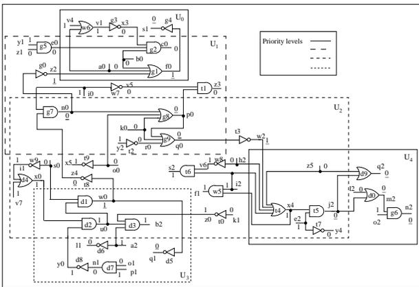
Figure 1: A digital circuit.
